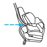
4. Insert the belt tongue into the proper buckle (the buckle closest to the direction the tongue is coming from) for that seating position until you hear a snap and feel the latch engage. Make sure the tongue is latched securely by pulling on it.
